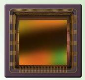
The CMV4000 is a high sensitivity, pipelined global shutter CMOS image sensor with 2048 x 2048 pixel resolution capable of HD format. Pipelining allows exposure during read out. The state-of-the-art pixel
