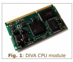
DIVA is a family of system-on-modules (SOM) that belongs to **DAVE Embedded Systems Lite Line** product class. DIVA is based on Texas Instruments "Sitara" AM335x Cortex-A8 application processor and is built with SO-DIMM 204 pin form factor.
