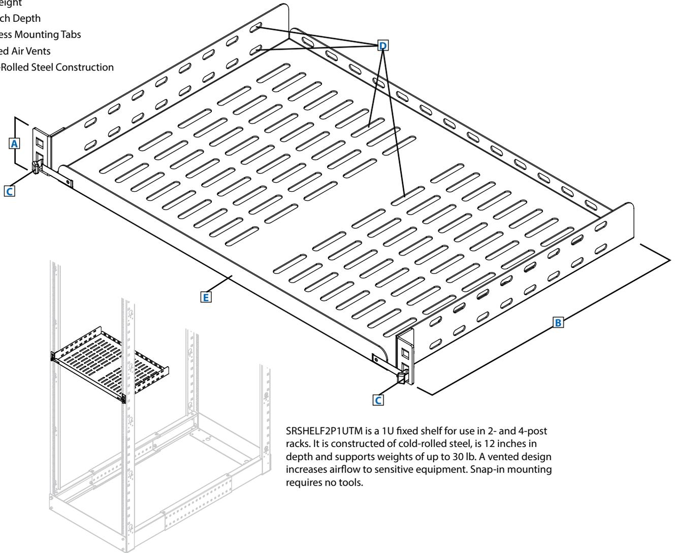
SRSHELF2P1UTM is a 1U fixed shelf for use in 2- and 4-post racks. It is constructed of cold-rolled steel, is 12 inches in depth and supports weights of up to 30 lb. A vented design increases airflow to sensitive equipment. Snap-in mounting requires no tools.
