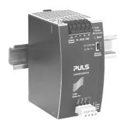
This buffer unit is a supplementary device for DC 24V power supplies and DC/DC converter. It delivers power to bridge typical mains failures or extends the hold-up time after turn-off of the AC or DC power. In times when the DC/DC converter provides sufficient voltages, the buffer unit stores energy in the integrated electrolytic capacitors. In case of mains voltage fault, this energy is released again in a regulated process.
