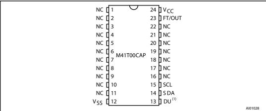
1. DU is "don't use". Do not connect. Must be allowed to float. Do not connect to  $V_{\text{CC}}$  or  $V_{\text{SS}}$ .
