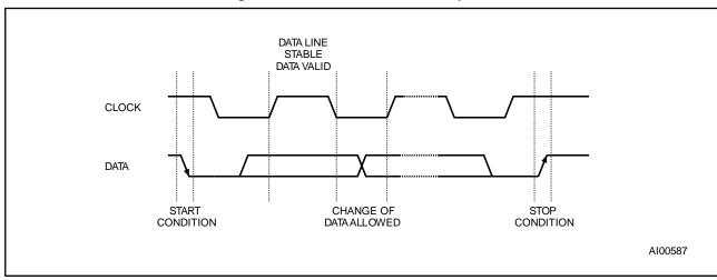
Figure 4: Serial bus data transfer sequence
