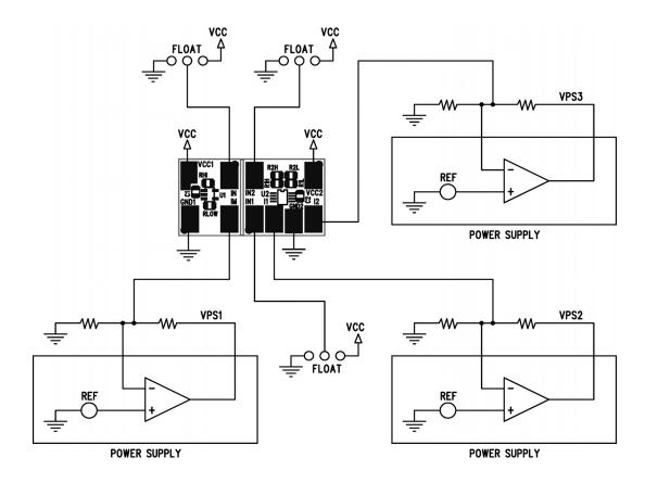
Figure 1. Proper Measurement Equipment Setup
