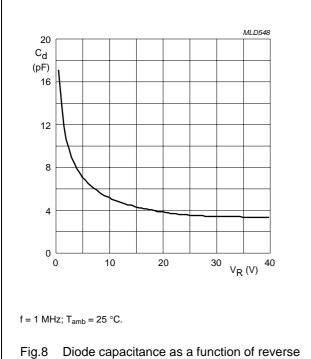
Fig.8 Diode capacitance as a function of reverse voltage; typical values.
