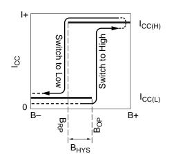
Figure 1. On the horizontal axis, the B+ direction indicates increasing south polarity magnetic field strength, and the B– direction indicates decreasing south polarity field strength (including the case of increasing north polarity).
