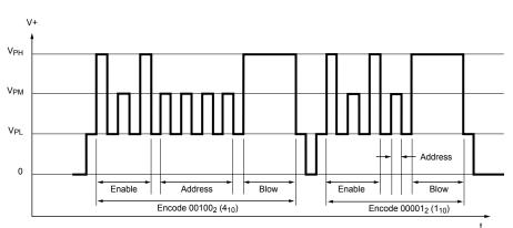
Figure 6. Pulse sequence to permanently encode calibration value 5 (101 binary, or bitfield address 3 and bitfield address 1).
