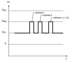
Figure 8. Pulse sequence to select addresses
