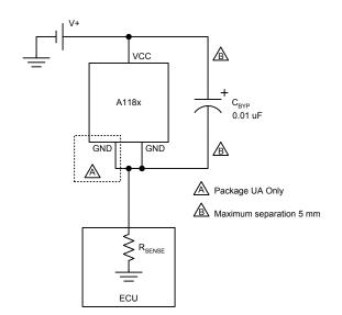
Figure 3. Typical application circuit
