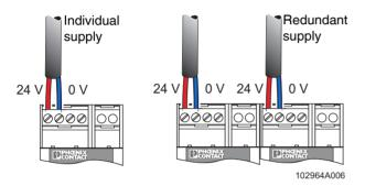
Figure 7 Individual/redundant supply
