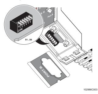
Figure 4 Setting the DIP switches
