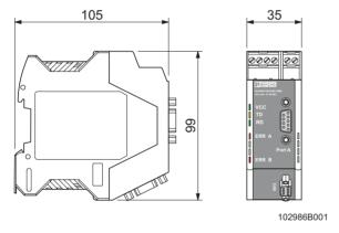
Figure 2 Housing dimensions (in mm)
