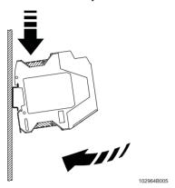
Figure 6 Assembly in the control cabinet
