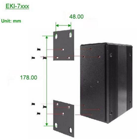
Figure 2.5: Combine the Metal Mounting Kit
