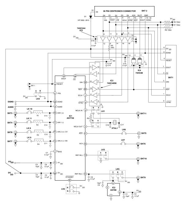
Figure 7. Evaluation Board Circuit Diagram
