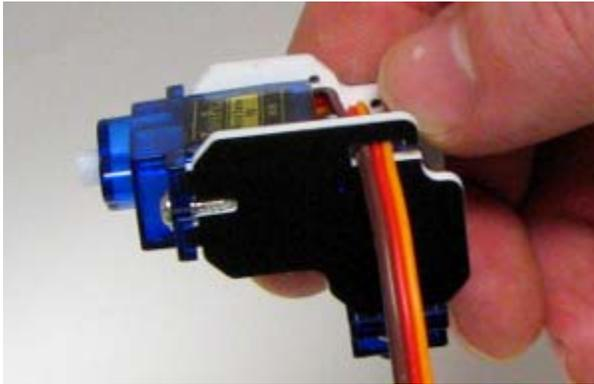
Tuck the servo wires through the holding slit on the mount plate D. The Servo head assembly is ready now.
