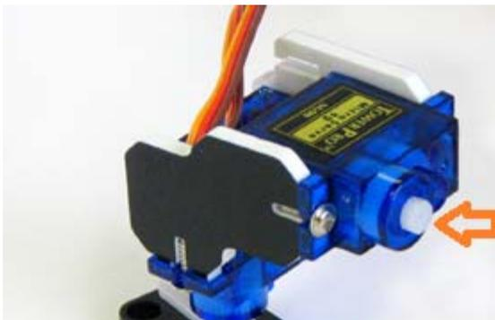
Note the servo on which the camera head will be mounted (Orange arrow).
