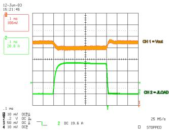
FIGURE 4. TRANSIENT WAVEFORM FROM 0A TO 52A
