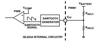
FIGURE 18. BATTERY VOLTAGE FEED-FORWARD COMPENSATION
