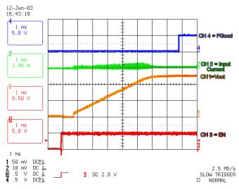
FIGURE 2. INRUSH CURRENT AT VIN 19V @ 52A
