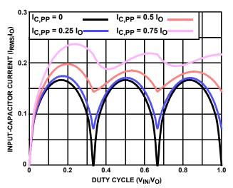
FIGURE 29. NORMALIZED INPUT-CAPACITOR RMS
