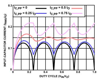
FIGURE 30. NORMALIZED INPUT-CAPACITOR RMS
