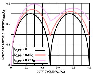
FIGURE 28. NORMALIZED INPUT-CAPACITOR RMS
