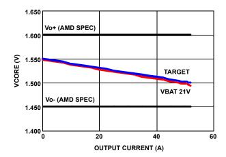
FIGURE 10. ISL6244 DROOP: V<sub>BAT</sub> = 21V
