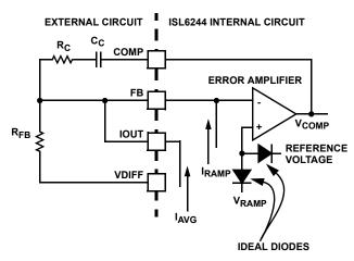
FIGURE 21. RAMP CURRENT AND VOLTAGE FOR REGULATING SOFT-START SLOPE AND DURATION
