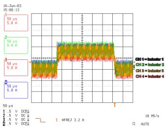
FIGURE 5. INDUCTOR CURRENT TRANSIENT
