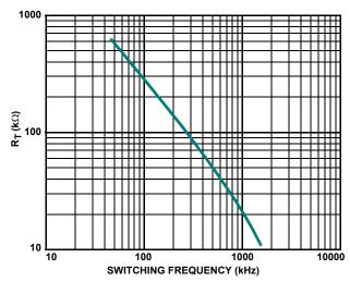
FIGURE 27. RT vs SWITCHING FREQUENCY
