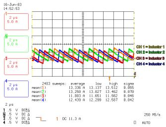
FIGURE 8. FOUR PHASE CURRENT BALANCE @ 52A
