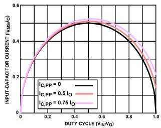
FIGURE 31. NORMALIZED INPUT-CAPACITOR RMS
