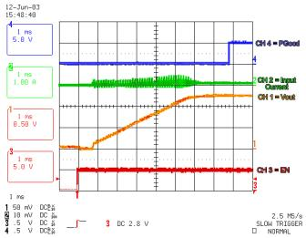
FIGURE 3. INRUSH CURRENT AT VIN 10.8V @ 52A
