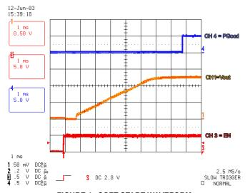
FIGURE 1. SOFT-START WAVEFORM
