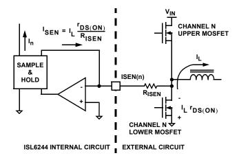
FIGURE 15. INTERNAL AND EXTERNAL CURRENT-SENSING CIRCUITRY
