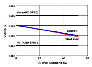
FIGURE 7. ISL6244 DROOP:  $V_{BAT} = 8.4V$
