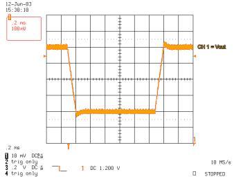
FIGURE 6. VID CHANGES FROM 1.60V TO 1.20V
