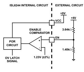
FIGURE 20. POWER SEQUENCING USING THRESHOLD-SENSITIVE ENABLE (EN) FUNCTION
