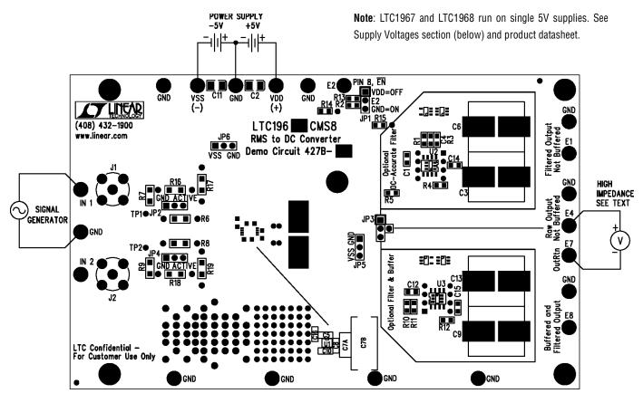
Figure 1. Proper Measurement Equipment Setup
