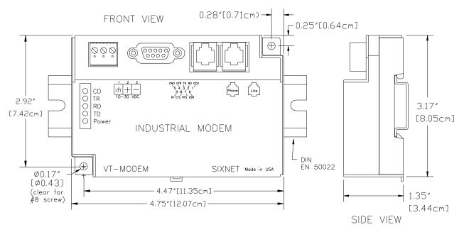
Figure 3-1: VT-MODEM DIMENSIONS, ALL MODELS
