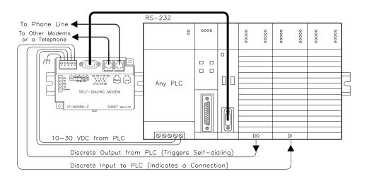
The Sixnet PLC Self-Dialing Modem (VT-MODEM-2) has all the features of the Sixnet Industrial Modem (VT-MODEM-1), plus the ability to dial out based on an alarm contact or PLC discrete output.
