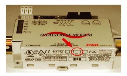
3. You can also detect the modem type using HyperTerminal. To query the firmware version enter **ati3<enter>**. Please see the tables below for information on how to interpret this firmware rev number.
