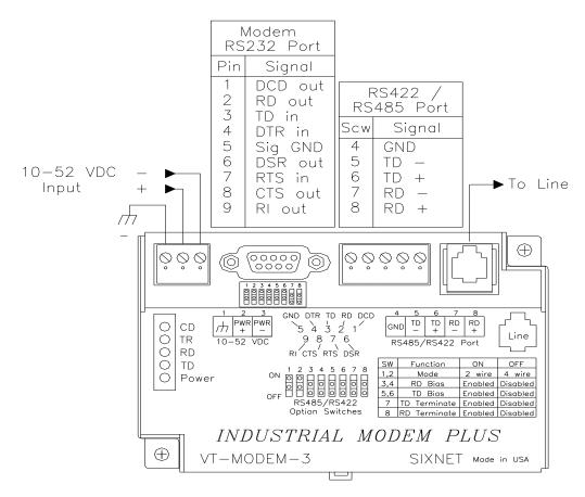
Figure 4-4: Typical RS422 / RS485 Wiring
