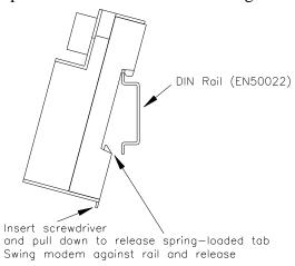
Figure 3-2: DIN RAIL MOUNTING
