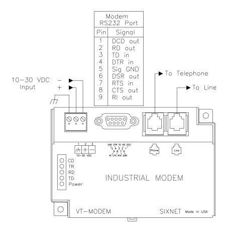
Figure 4-2: VT-MODEM-1 WIRING
