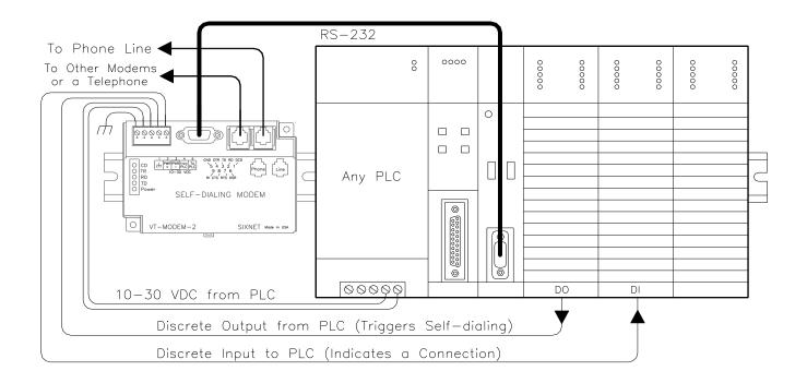
Figure 4-3: VT-MODEM-2 WIRING
