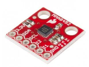
The MMA8452Q is just a solid 3-axis accelerometer. It supports three, selectable sensing ranges:  $\pm$  2g, 4g, or 8g. It sports features like orientation detection, single and double-tap sensing, and low power modes. It's a
