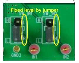
Jumper indicated on the left is adopted on this evaluation board to set operation of the TB6642FG. To select the function by the jumper, supply the voltage of high level by VDD pin.
