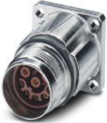
Device connector, front mounting, straight, SPEEDCON locking, M17, Number of positions: 8, Type of contact: Socket, Crimp connection, Axial O-ring, 4xØ2,7, shielded: yes, Flange dimensions: 21.6 mm x 21.6 mm
