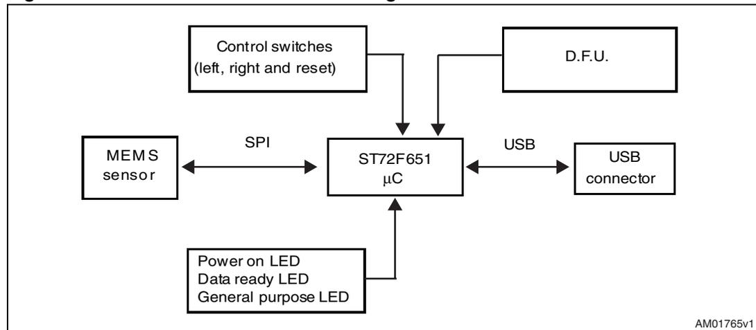
The ST7-USB microcontroller included on the board allows communication between the sensor device and the PC. The user can interact with the hardware either through the GUI provided with the kit or through dedicated software routines to run customized applications.
