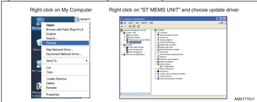
Figure 7. USB driver installation using the hardware update wizard
