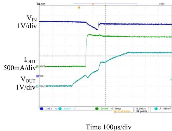
Figure 25. Leave OVP Function ( $V_{IN}=6V$  to  $5V$ )
