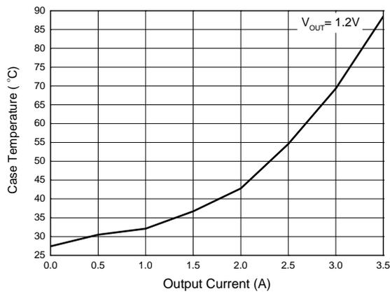
Figure 14. Case Temperature vs. Output Current
