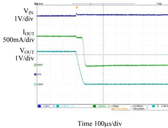
Figure 24. OVP Function ( $V_{IN}=5V$  to  $6V$ )
