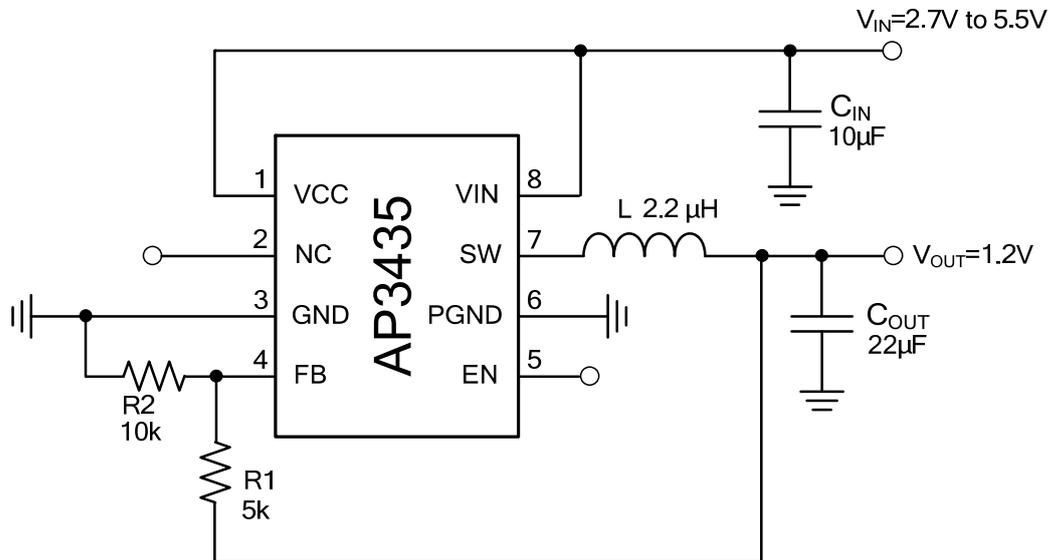
Note 2:  $V_{OUT} = V_{REF} \times \left(1 + \frac{R_1}{R_2}\right)$ .
