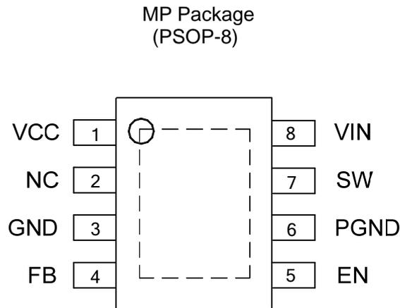
Figure 2. Pin Configuration of AP3435 (Top View)
