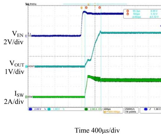
Figure 15. Enable Waveform
