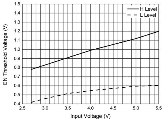
Figure 12. Enable Threshold Voltage vs. Input Voltage
