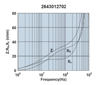
Impedance, reactance, and resistance vs. frequency.
