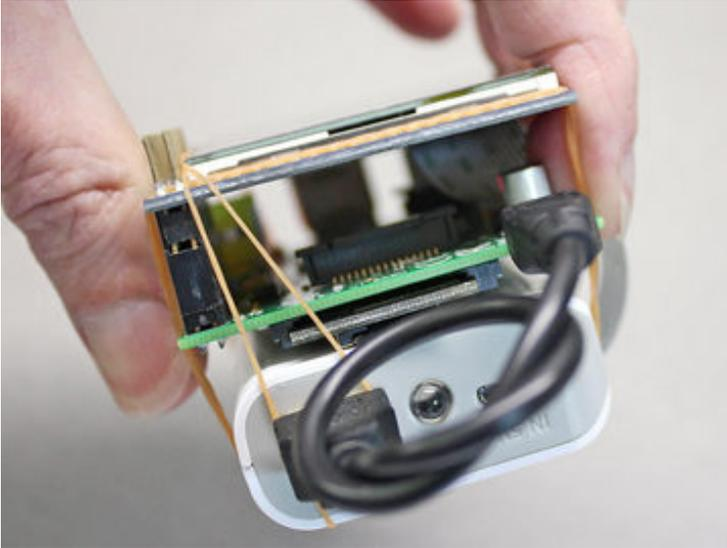
makers could squeeze a slim LiPo battery and a 5V boost converter in there, connecting to the expansion header at the right edge of the TFT board instead of the side-protruding USB power connector. The result would be similar in size to some consumer point-and-shoot digital cameras.
