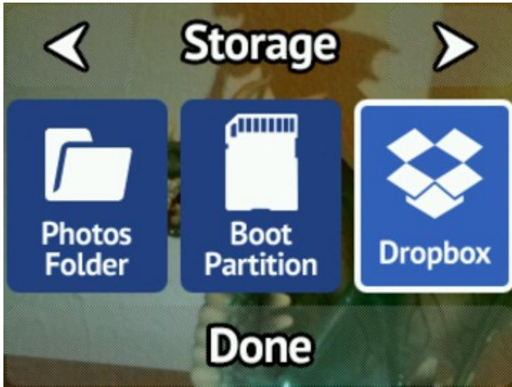
be saved inside a “Photos” folder in your Raspberry Pi home directory (the folder will be created if it doesn’t exist). They can be easily accessed from other programs on the Pi, but this partition isn’t easily accessed when inserting the SD card in other computers.
