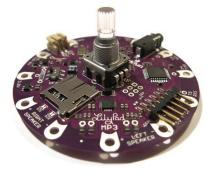
• Insert the Rotary Encoder's pins into the holes in the center of the LilyPad MP3 Player. Note that it goes into the "top" side of the board (the side with the silkscreen that indicates where the encoder goes).
