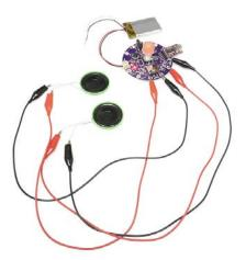
The LilyPad MP3 Player comes with preinstalled software called **"Trigger"** that will play specific files when the input pins are grounded. You can also add an optional rotary encoder and load the **"Player"** software to turn the board into a "real" audio player, or even write your own software using the free Arduino programming environment.
