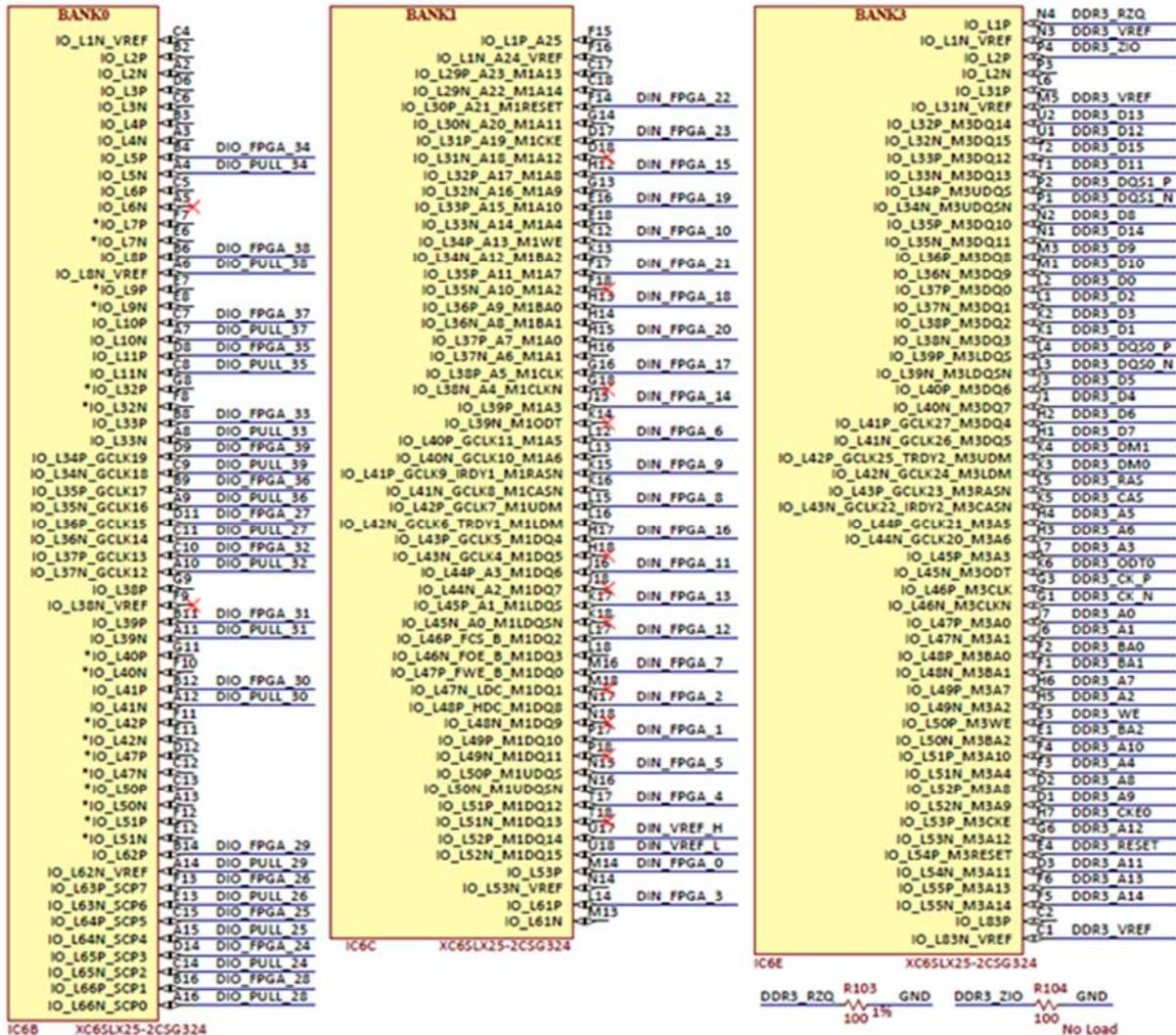
Figure 21. FPGA banks 0, 1 and 3.
