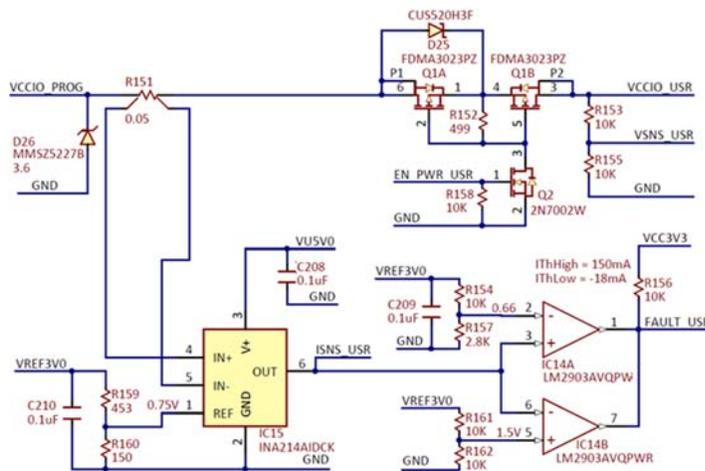
Figure 14. VCCIO\_USR protection and switch.
