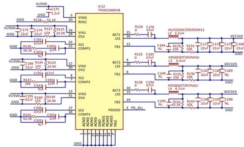
Figure 12. Internal voltage supplies.
