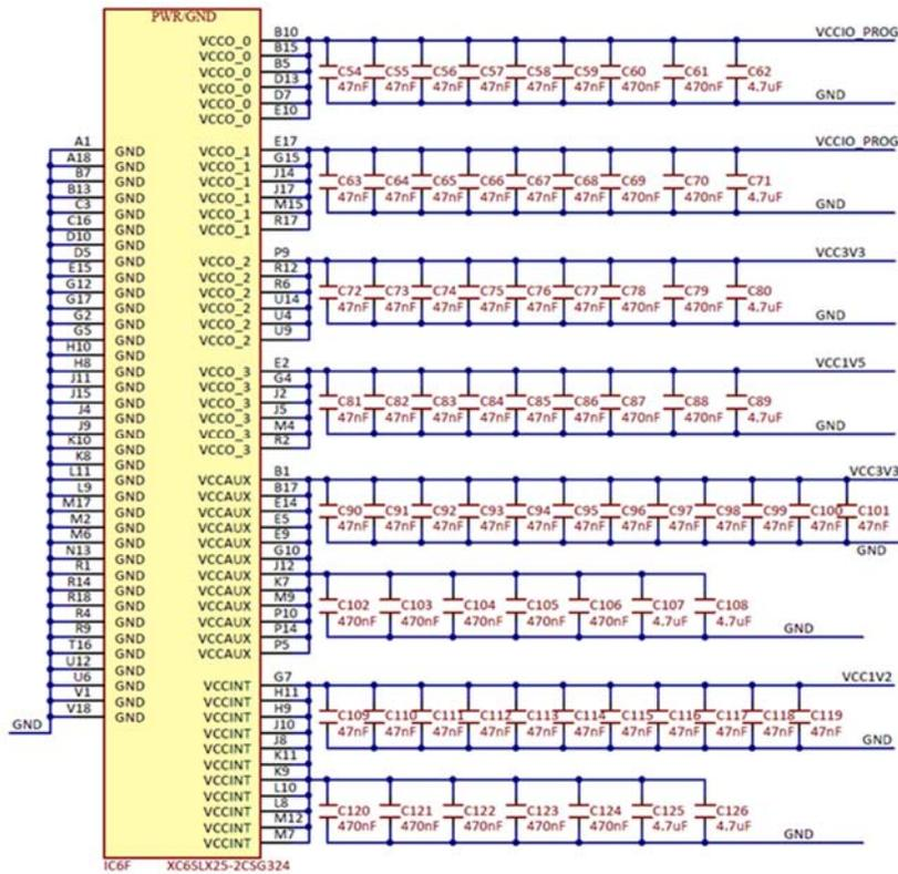
Figure 22. FPGA powering and decoupling.
