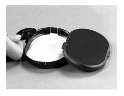
4.2 Peel the backing from the multimode (light green) polishing paper and stick it to the polishing pad surface. One sheet of polishing paper can polish two connectors.
