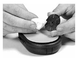
4.5.2 Moisten the singlemode polishing film with a little water and place the singlemode (pale yellow) film, shiny side down, on top of the singlemode polishing film.
