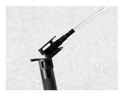
3.16 For 3M™ Crimplok™ SC Connector: Crimp only the end of the smaller diameter of the crimp ring with the .137" cavity of the crimp tool to the 3 mm jacket. Do not crimp the middle portion of the crimp ring.
