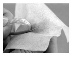
3.6 For 3M™ Crimplok™ SC Connector only: Insert the fiber through the connector until the jacket bottoms out on the connector. The fiber will form a gentle bend, resting in the fiber support groove.
