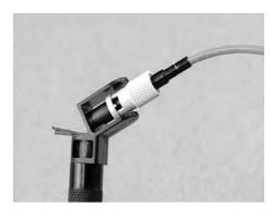
3.14 Crimp the large diameter section of the crimp ring with the .190" cavity of the crimp tool.
