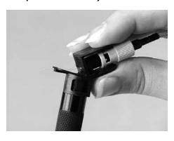
3.18 Press the connector forward to ensure that the ferrule is still seated against the stop.
