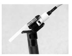
3.20 SLOWLY depress the button on the activation tool until the fiber breaks away.
