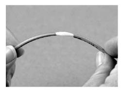
3.4 For Crimplok SC connector: Strip fiber. Leave 3/8 to 1/2 inch (9 to 12 mm) of buffer protruding from jacket.
