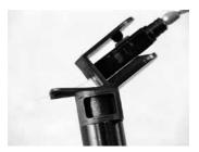
3.7 For Crimplok SC connector only: While holding the aramid yarn and the activation tool in one hand, load the gold sleeve of the connector into the .120" cavity of the crimp tool. Partially close the crimp tool to secure the connector.
