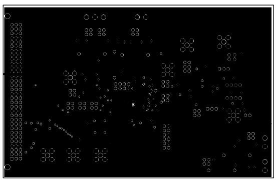
Figure 11. Inner Layer Ground Planes
