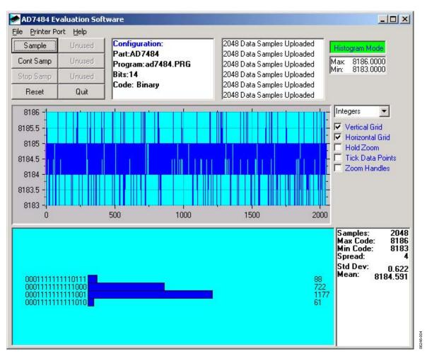
Figure 4. AD7484 Main Window – Histogram Mode
