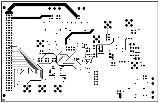
Figure 14. Bottom Layer Etch
