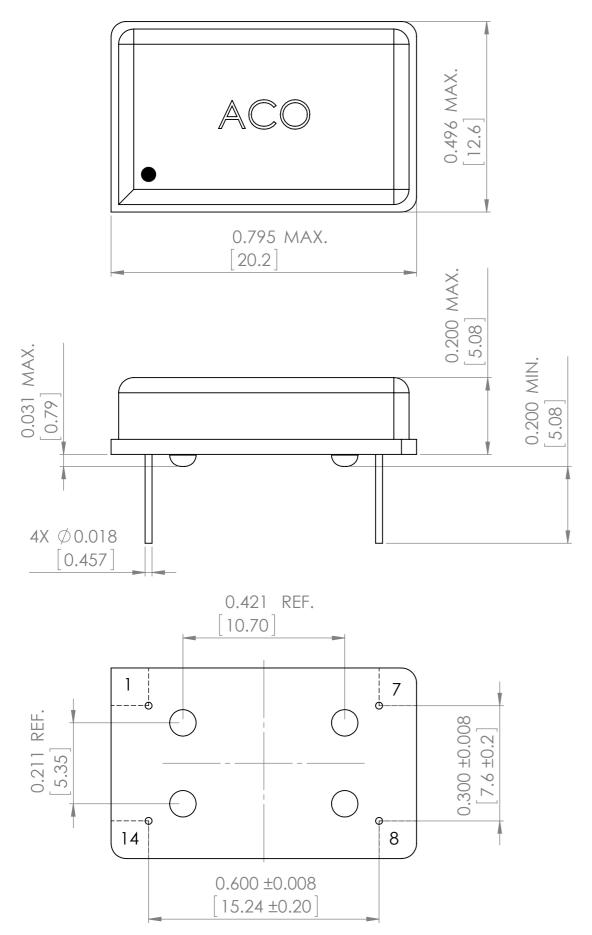
The height of the package vary depending on the frequency >100MHz. Please contact ABRACON for the height information for F>100MHz.
