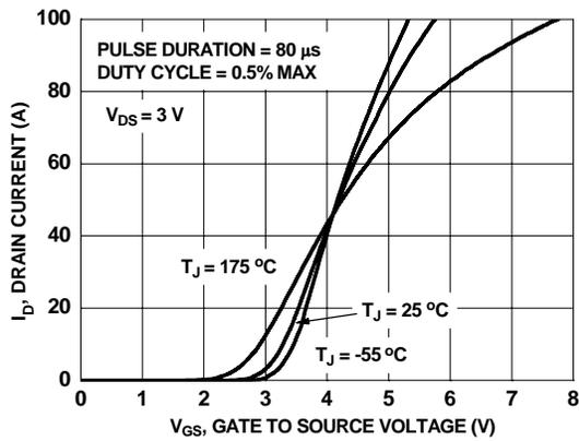
**Figure 5. Transfer Characteristics**
