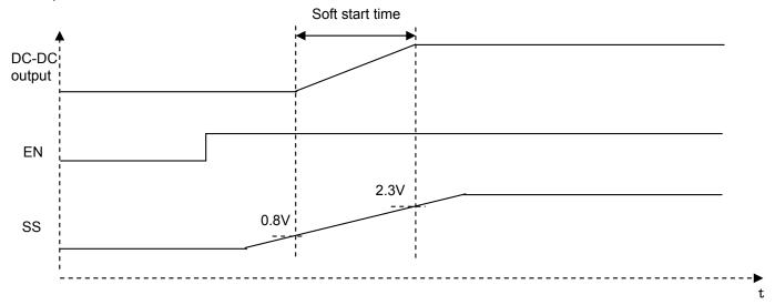
Figure: Soft start operation timing chart
