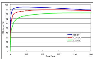
Condition )  $\label{eq:Vin} \mbox{Vin = 6 , 12 , 25 V, Vout = 5 V,} \\ \mbox{Lo = 10 } \mbox{\mu H, Co = 22 } \mbox{\mu F, Frequency = 490 kHz} \\ \mbox{RSENSE=50m} \ \Omega$
