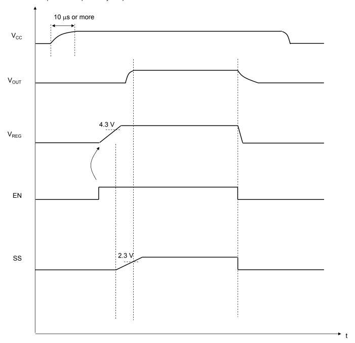
Figure: Power ON/OFF sequence by EN
