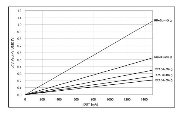
Figure :  $\Delta$ = Vout – V\_USB vs IOUT
