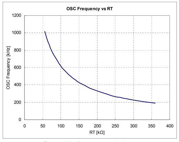
Figure: switching frequency vs external resistance
