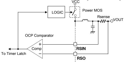
Figure: Over-Current Protection circuit block diagram
