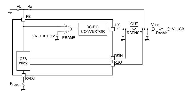
Figure: The diagram of current feed back function
