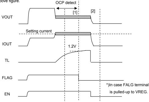
Figure : Method of detection of Over-Current Protection function
