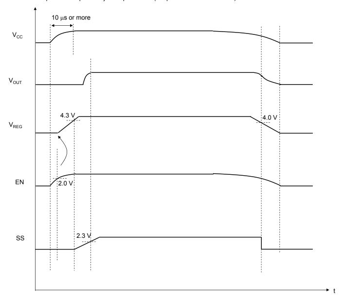
Figure: Power ON/OFF sequence by VCC/EN
