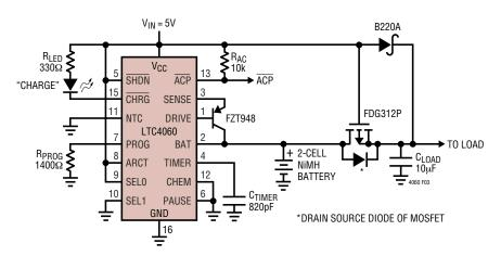
Figure 3. 1A Charger Application with Power Path Control
