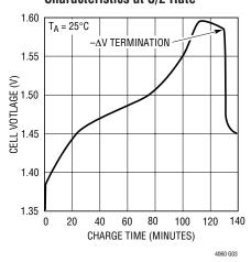
NiCd Battery Charging Characteristics at C/2 Rate
