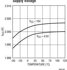
I<sub>FCL</sub> vs Temperature and Supply Voltage
