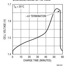
NiMH Battery Charging Characteristics at C/2 Rate
