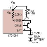
Figure 5. Extended Charge Current Operation
