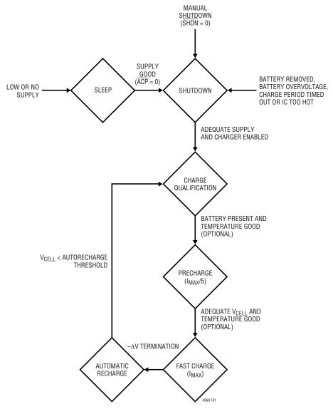
Figure 1. LTC4060 Basic State Diagram
