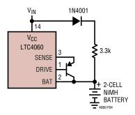
Figure 4. Adding Trickle Charge
