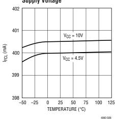
I<sub>BRD</sub> vs Temperature and Supply Voltage
