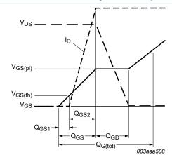
Fig. 13. Gate charge waveform definitions
