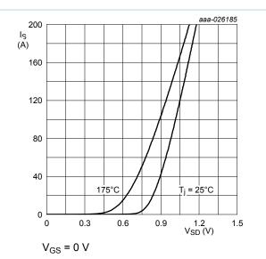
function of source-drain (diode forward) voltage; typical values
