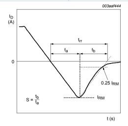
Fig. 16. Reverse recovery timing definition
