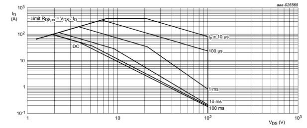
T<sub>mb</sub> = 25 °C; I<sub>DM</sub> is a single pulse
