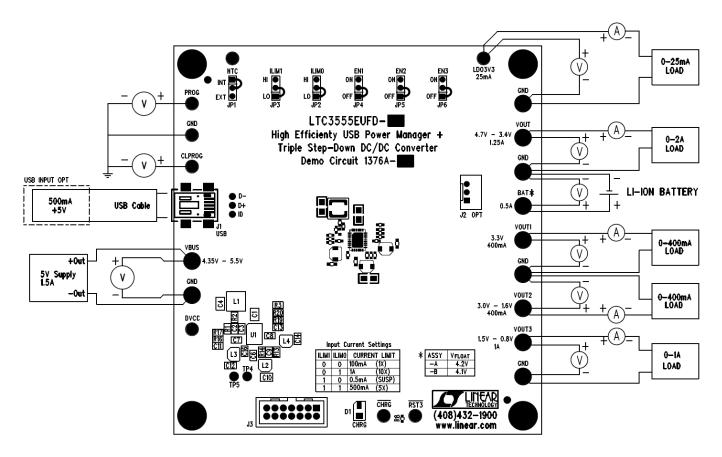
Figure 2. Proper Measurement Equipment Setup
