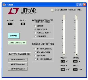
Figure 1. Graphical User Interface Demonstration Software for DC1376A-A and DC1376A-B.
