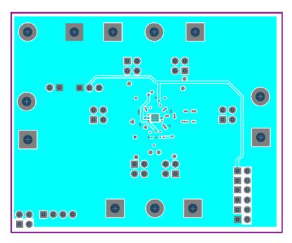
**Evaluation Board Layer – Layer 5 (V<sub>IN</sub> Plane)**
