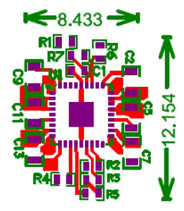
**Evaluation Board Top Layer - Power Component Placement**
