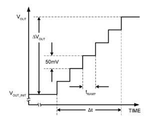
Figure 8. Buck DVC Control Ramp
