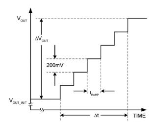
Figure 12. Boost DVC Control Ramp
