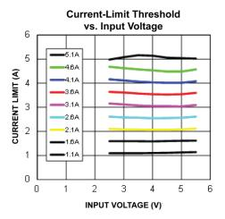
Figure 13. Current-Limit Threshold vs. Input Voltage
