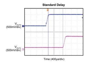
Figure 14. Standard Delay Time
