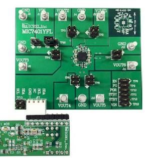
Figure 2. USB Dongle Connection to Evaluation Board
