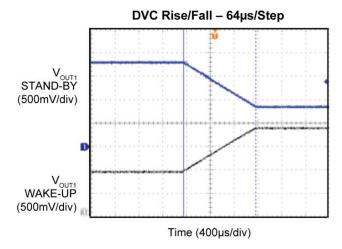
Figure 9. Buck DVC Control Ramp
