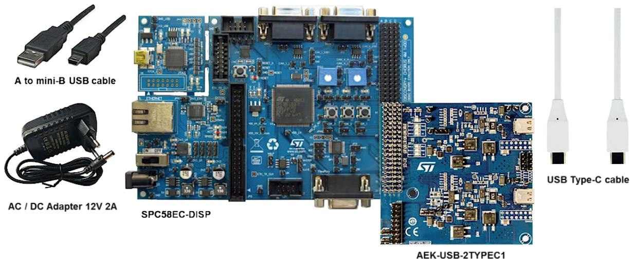
The [AEK-USB-2TYPEC1](#) interface board hosts a pair of [STUSB1702Y](#) automotive grade USB Type-C controllers; one for each USB Type-C port. The board contains a dual Transil™ array [ESDA25LY](#) and very low capacitance [USBLC6-2SC6Y](#) devices for ESD protection. The status of the ports is signaled on the board through a set of LEDs for each port. The board includes about 20 test points.
