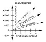
current change. The input summing resistor values are weighted in a binary progression, so they can be switched in combinations to give 32 discrete steps of span. The fine adjust control brackets these coarse steps and can be adjusted to the exact span needed.
