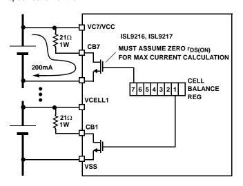
FIGURE 7. CELL BALANCING CONTROL EXAMPLE WITH 100mA BALANCING CURRENT
