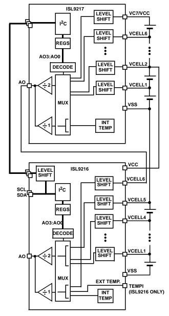
FIGURE 6. ANALOG OUTPUT MONITORING DIAGRAM
