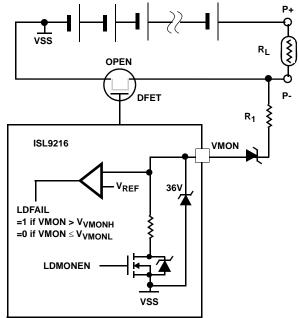
FIGURE 4. LOAD MONITOR CIRCUIT
