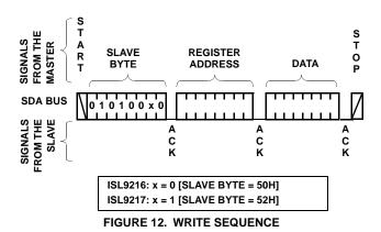
When receiving data from the master, the value in the data byte is transferred into the register specified by the address byte on the falling edge of the clock following the 8th data bit.
