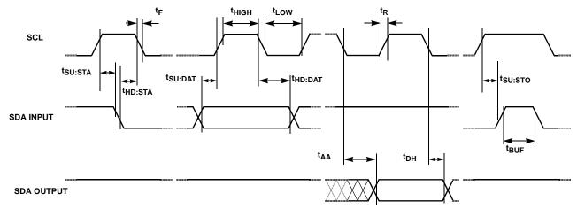
This timing shows the communication with the ISL9216. Communication with the ISL9217 (through the ISL9216) adds some lag time, however, overall the communication with the ISL9217 meets the same timing requirements as communication with the ISL9216.
