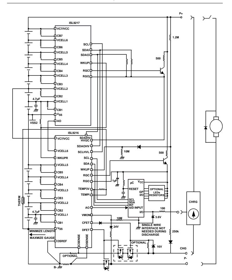
FIGURE 18. 12-CELL CASCADED APPLICATION CIRCUIT WITH SEPARATE CHARGE/DISCHARGE
