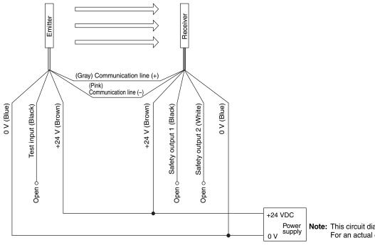
**Note:** This circuit diagram is used for operation check. For an actual circuit example, refer to page 23.
