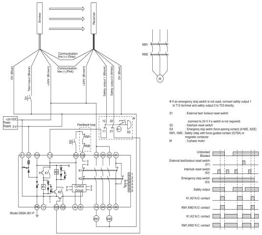
Note: 1. As the G9SP Safety Controller is a PNP output type, it cannot be connected to the F3SJ-E□□□□N25. Also, a Safety Controller with PNP output cannot be connected to the F3SJ-E□□□□N25.
