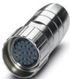
Cable connector, straight, Screw locking, M27, number of positions: 26, type of contact: Socket, Crimp connection, shielded: yes, cable diameter range: 2 mm ... 14.5 mm
