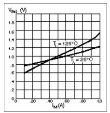
Figure 11. Typical source saturation vs. output current
