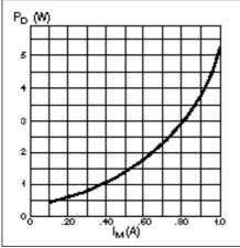
Figure 15. Typical power dissipation vs. motor current
