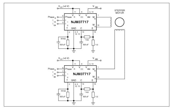
Figure 8. Typical stepper motor driver application with NJM37717
