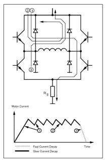
Figure 5. Output stage with current paths for fast and slow current decay
