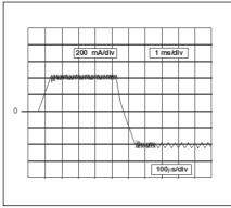
Figure 4. Motor current (I<sub>M</sub>), Vertical: 200 mA/div, Horizontal: 1 ms/div, expanded part 100 µs/div
