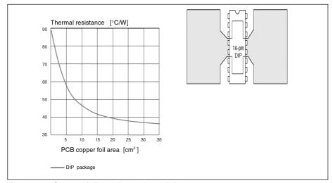
Figure 10. Copper foil used as a heatsink
