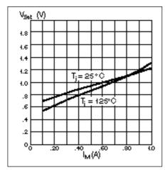
Figure 12. Typical sink saturation vs. output current
