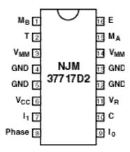
Figure 2. Pin configurations
