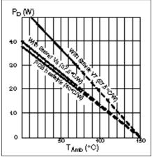
Figure 16. Allowable power dissipation vs. ambient temperature
