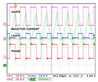
FIGURE 12. SWITCHING WAVEFORMS IN CONTINUOUS CONDUCTION MODE
