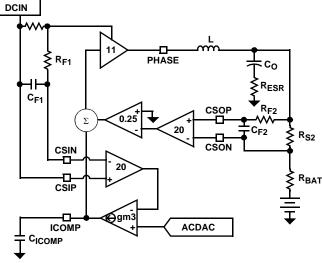
FIGURE 25. ADAPTER CURRENT LIMIT LOOP
