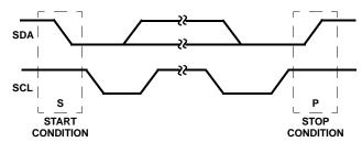
FIGURE 16. START AND STOP WAVEFORMS
