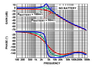
FIGURE 20. FREQUENCY RESPONSE OF THE LC OUTPUT FILTER
