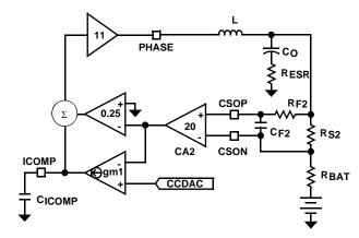
FIGURE 23. CHARGE CURRENT LIMIT LOOP
