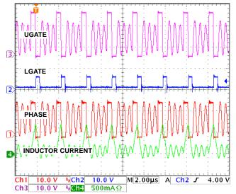
FIGURE 11. SWITCHING WAVEFORMS IN DISCONTINUOUS CONDUCTION MODE
