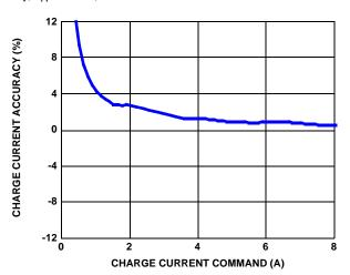
FIGURE 4. CHARGE CURRENT ACCURACY
