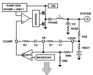
FOR SMALL SIGNAL AC ANALYSIS, VOLTAGE SOURCES ARE SHORT CIRCUITS AND CURRENT SOURCES ARE OPEN CIRCUITS.
