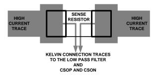
FIGURE 26. CURRENT SENSE RESISTOR LAYOUT
