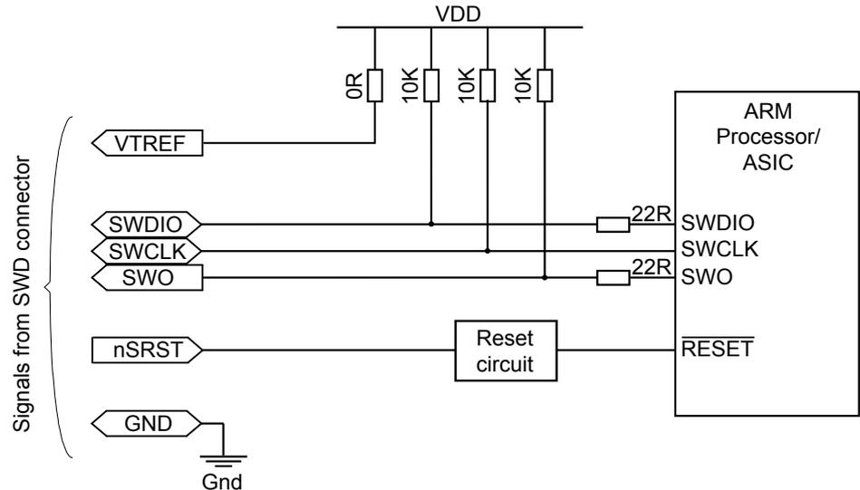
Figure 2-3 Typical SWD connections
