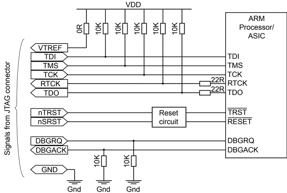
Figure 1-3 Typical JTAG connection scheme
