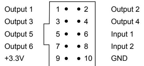
**Figure 3-1 USER I/O connector pinouts**
