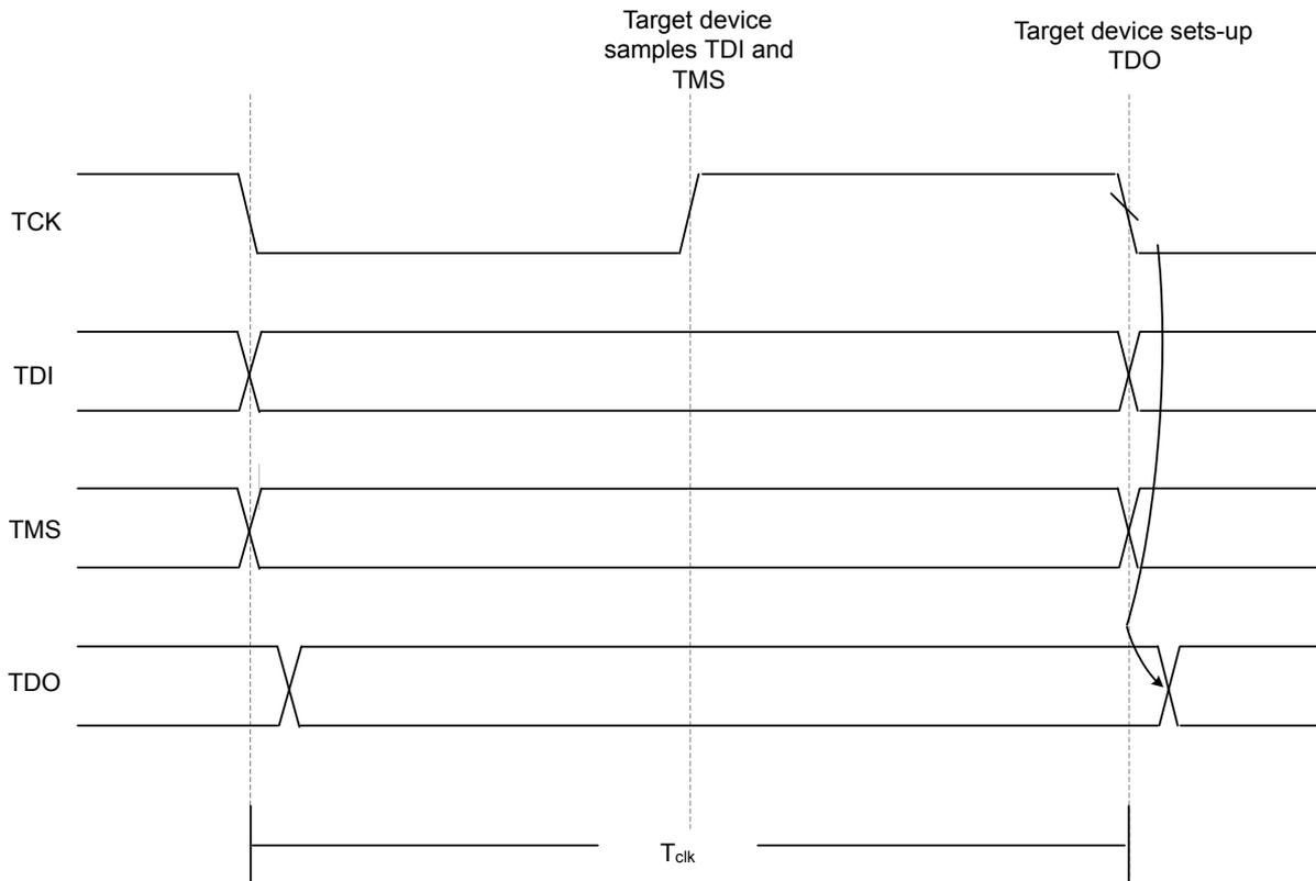
**Figure 2-6 JTAG port timing diagram**
