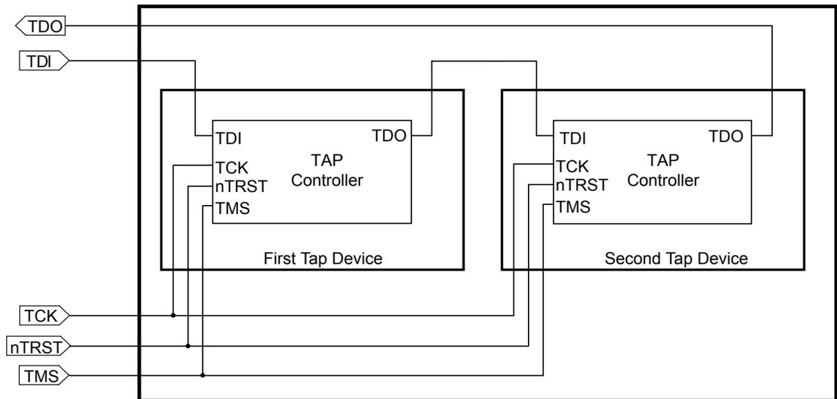
**Figure 1-2 TAP Controllers serially chained within an ASIC**
