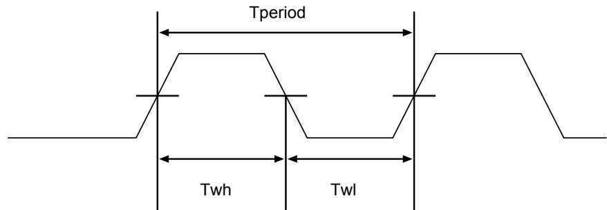
Figure 2-5 Clock waveforms
