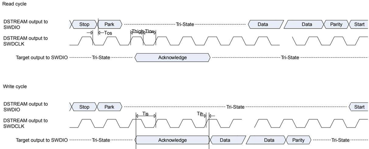
**Figure 2-4 SWD timing diagrams**
