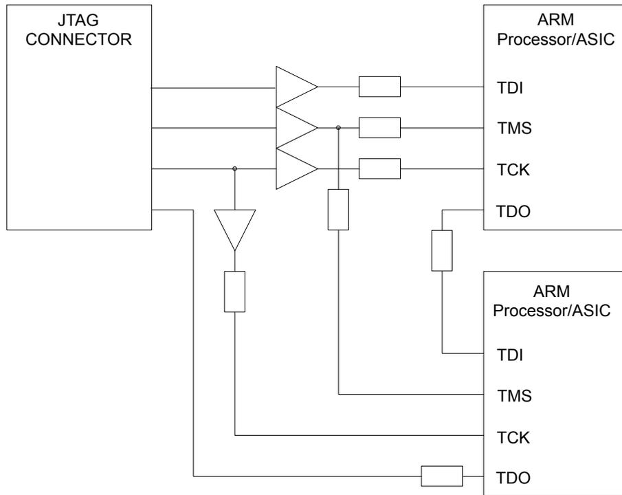
**Figure 2-11 JTAG connection with de-skewed buffers**
