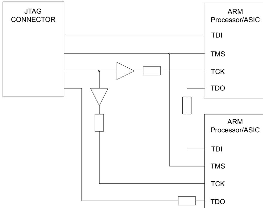
**Figure 2-10 Daisy-chained JTAG connection with TCK buffers**
