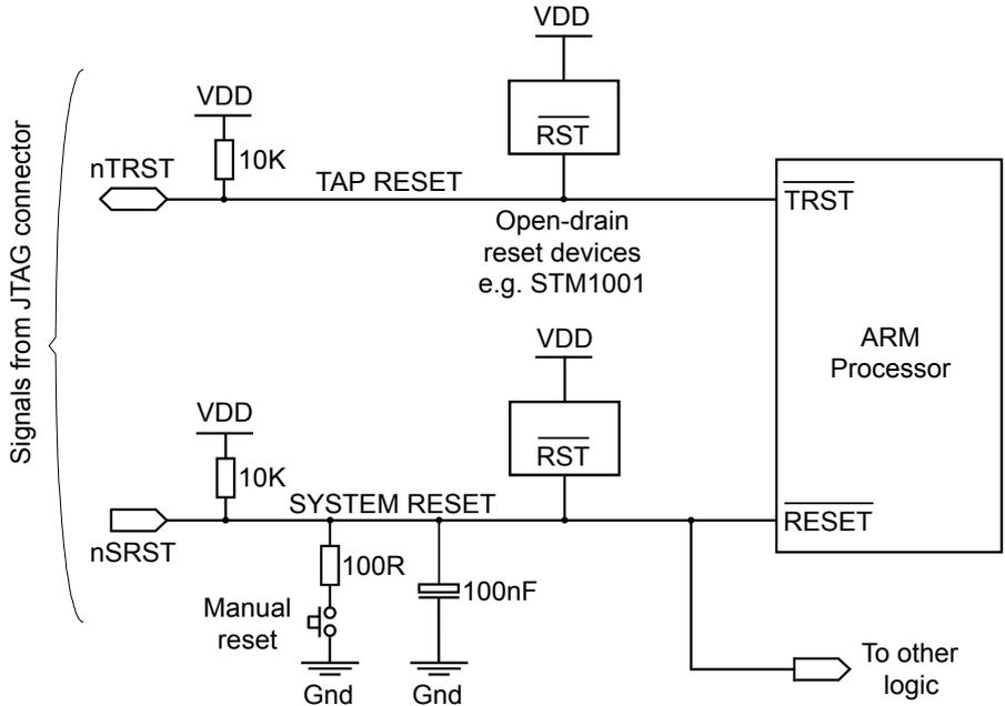
Figure 1-1 Example reset circuit logic
