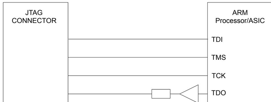
**Figure 2-8 JTAG connection with TDO buffer**
