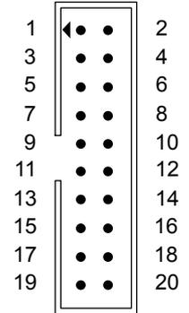
Figure 2-1 ARM JTAG 20 connector pinout
