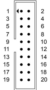
Figure 2-2 CoreSight 20 connector pinout
