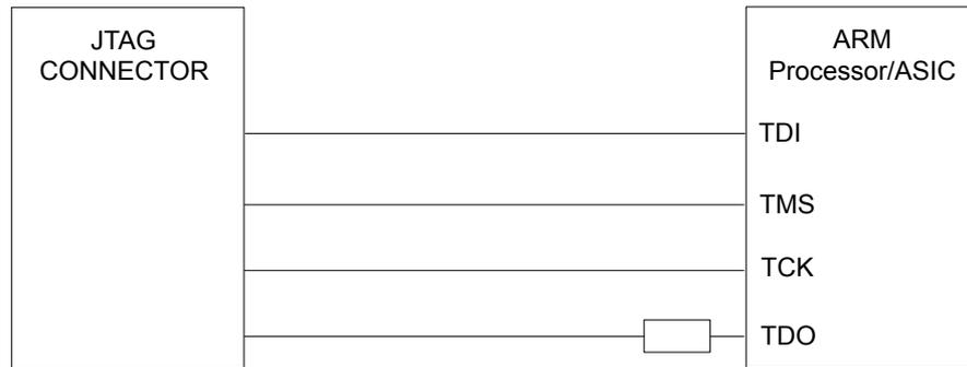
**Figure 2-7 JTAG connection without buffers**
