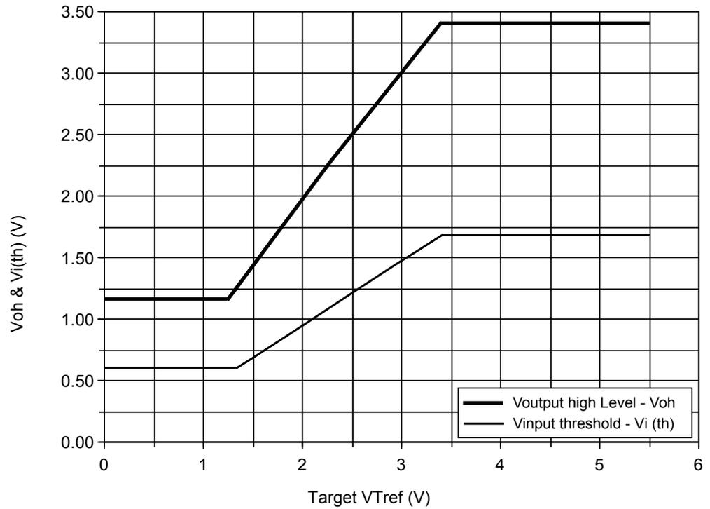
**Figure 1-4 Target interface logic levels**
