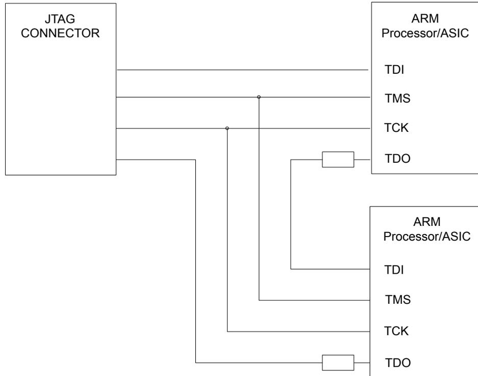
**Figure 2-9 Daisy-chained JTAG connection without buffers**
