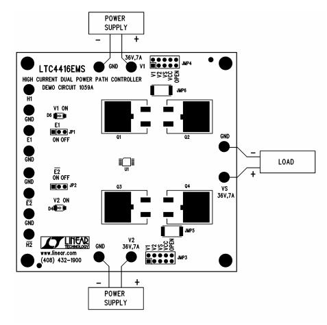
Figure1: Proper Measurement Equipment Setup
