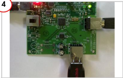
To connect to the PC, plug the USB A to B cable into the hub's 'Up Stream' connector P1. Plug the other end of the cable into one of the PC's host controller ports. The hub enumerates as a 'Generic USB Hub'. The hub is now ready for any low speed, full speed, or high speed devices to be plugged into the ports. For the 2-port hub, the board is labeled PORT1 and PORT2.
