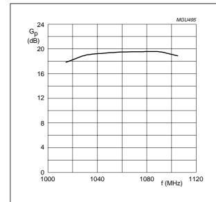
$T_h$  = 25 °C;  $V_{DS}$  = 36 V;  $I_{DQ}$  = 50 mA; class-AB;  $P_L$  = 10 W;  $t_p$  = 50  $\mu s; \, \delta$  = 2%.
