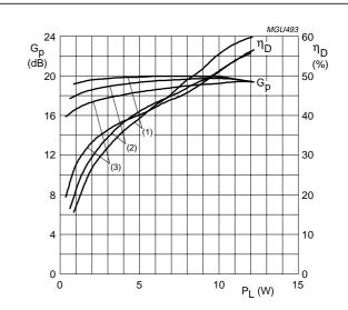
$T_h$  = 25 °C;  $V_{DS}$  = 36 V;  $I_{DQ}$  = 50 mA; class-AB;  $t_p$  = 50  $\mu s;$   $\delta$  = 2%.
