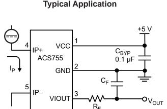
Application 1. The ACS755 outputs an analog signal,  $V_{OUT}$ . that varies linearly with the unidirectional DC primary sensed current,  $I_P$ , within the range specified.  $C_F$  is recommended for noise management, with values that depend on the application.
