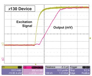
Step Response 50 A Excitation Signal, T<sub>A</sub>=25°C
