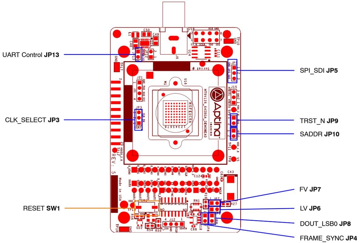
Figure 3. Top View of Evaluation Board – Jumpers
