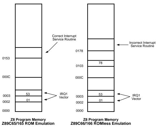
**Note:** The Incorrect Vectored Interrupt emulation only applies to the emulator. The Z89C66/166 device does not exhibit this problem.
