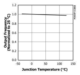
Figure 24. Output Frequency vs. Junction Temperature.
