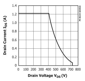
Figure 17. Maximum Allowable Drain Current vs. Drain Voltage.
