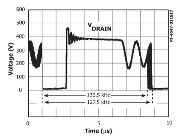
Figure 5. Frequency Jitter.
