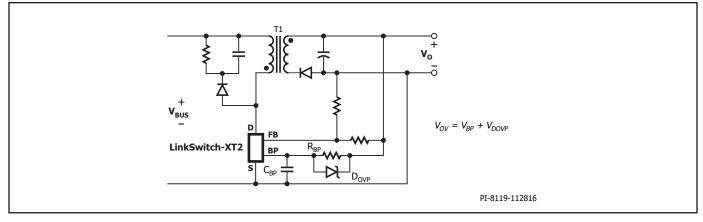
Figure 6. Non-Isolated Flyback Converter with Output Overvoltage Protection.
