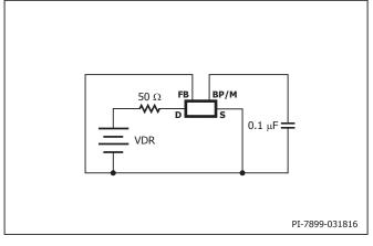
Figure 13. LinkSwitch-XT2 Duty Cycle Measurement.
