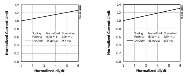
Figure 22. Default Current Limit vs. di/dt.
