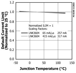
Figure 20. Default Current Limit vs. Junction Temperature.
