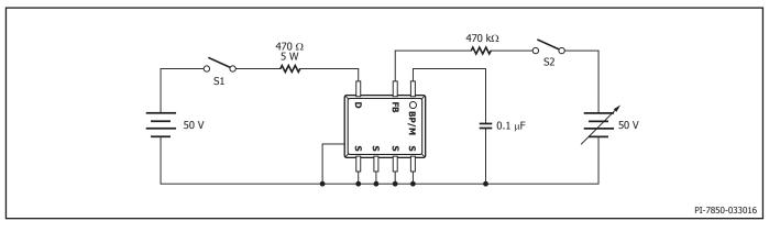
Figure 12. LinkSwitch-XT2 General Test Circuit.
