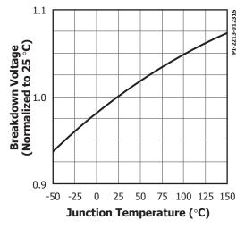
Figure 16. Breakdown vs. Temperature.
