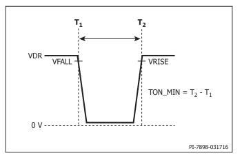
Figure 15. LinkSwitch-XT2 Minimum On-Time Measurement.
