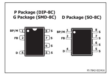
Figure 4. Pin Configuration.
