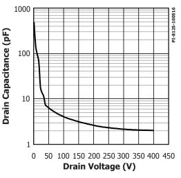
Figure 19. C<sub>oss</sub> vs. Drain Voltage.
