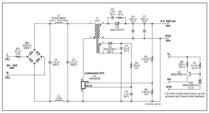
Figure 8. 2.5 W Universal Input Design using LNK3604.
