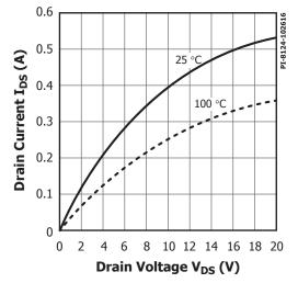
Figure 18. Output Characteristics.
