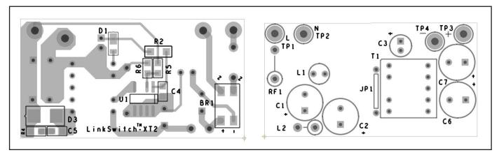
Figure 9. Recommended Printed Circuit Layout for LinkSwitch-XT2 using D Package in a Flyback Converter Configuration (Bottom Left, Top Right).
