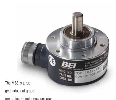
viding a unique combination of performance and flexibility. The M58 features a wide range of resolutions, up to 80,000 cycles per turn. The robust design of the M58 provides it with excellent resistance to shock and vibration. IP65 environmental protection level is standard (or IP67 is available with sealing flange). The M58 is an ideal replacement encoder for metric equipment used in many industries in the US.
