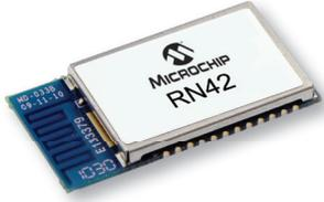
The RN42 Bluetooth Classic module has a 3 Mbps data rate for distances up to 20 meters and the RN41 has a range of up to 100 meters. Offering a small form factor and complete on-board package, these modules are ideal for applications ranging from basic cable replacement to barcode scanners, medical devices and computer accessories.
