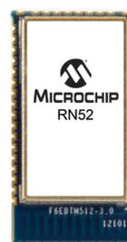
The RN52 audio module is a fully integrated solution for delivering high-quality stereo audio in a small form factor. This low-power audio module easily pairs with any smartphone, streams music and takes hands-free calls. It has many applications including wireless stereo speakers and headsets, wireless audio docking stations for smartphones, smartphone app streaming and more.
